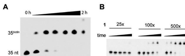
**Fig. 2** (A) A time course experiment with  $1.7 \text{ mM}$  tetrazine (samples taken after 0 min, 5 min, 10 min, 20 min, 30 min, 1 h and 2 h). After 10 minutes almost all of the starting material is consumed. (B) Effect of the excess of tetrazine on the reaction speed. 25 (25 $\times$ ,  $22 \mu\text{M}$ ) to 500 fold excess (500 $\times$ ,  $450 \mu\text{M}$ ) of tetrazine was added. The reactions were stopped after different time points (5 min, 10 min, 30 min, 1 h, and 2 h).
