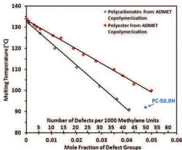
Fig. 7 Peak melting points of random long spaced polycarbonates (blue) and polyesters (red) for comparison<sup>34</sup> vs. the mole fraction of defect groups (carbonate groups or ester groups, respectively).
