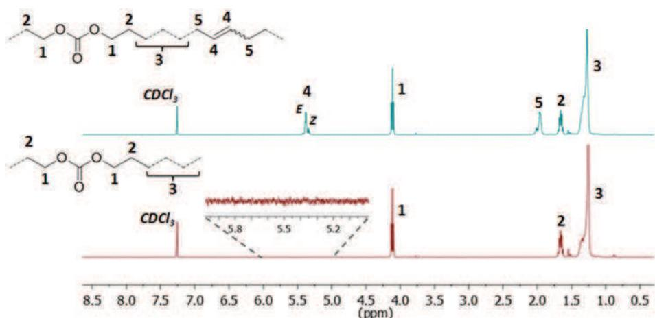
Fig. 4 <sup>1</sup>H NMR spectra of the unsaturated polycarbonate PC-42.9 (top, CDCl<sub>3</sub>, 400 MHz, 25 °C) and the corresponding saturated polycarbonate PC-42.9H (bottom, CDCl<sub>3</sub>, 400 MHz, 25 °C).
