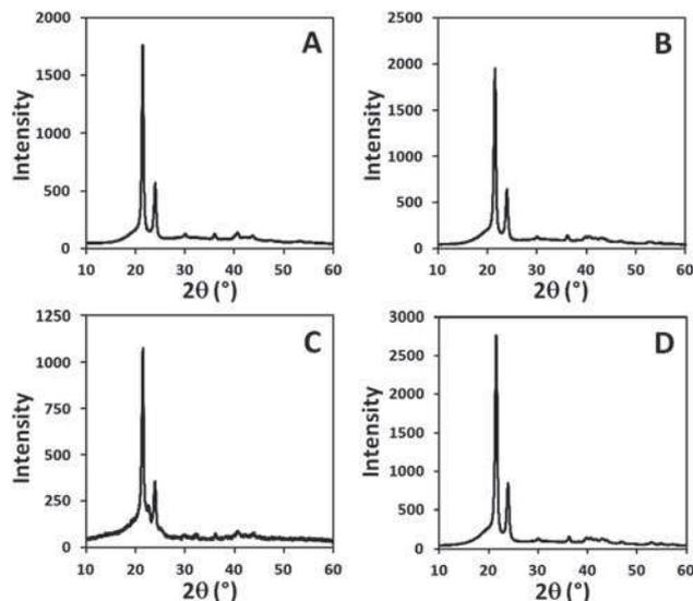
**Fig. 6** WAXD diagrams of random long chain polycarbonates **PC-37.5H** (A) and **PC-5.5H** (B), regular spaced polycarbonate **PC-19** (C) and defect free linear polyethylene **PC-0.0H** (D) from ADMET polymerization.
