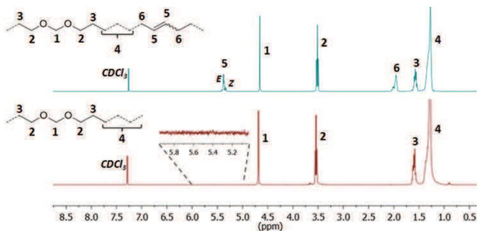
Fig. 3 <sup>1</sup>H NMR spectra of the unsaturated polyacetal PA-50.0 (top, CDCl<sub>3</sub>, 400 MHz, 25 °C) and the corresponding saturated polyacetal PA-50.0H (bottom, CDCl<sub>3</sub>, 400 MHz, 25 °C).
