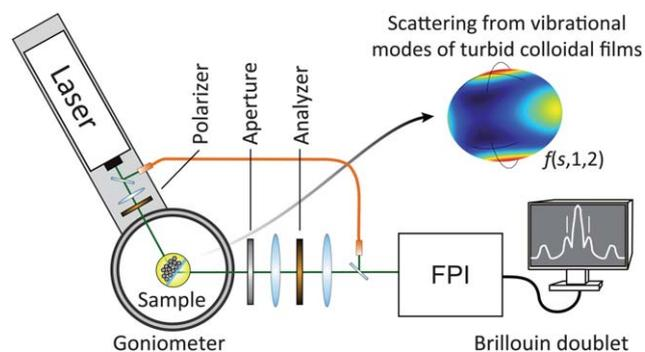
**Fig. 2** Scheme of BLS instrumentation. A single-mode laser (532 nm) illuminates the turbid film and multiply scattered light is analyzed by a FP interferometer. The observed frequency shift represents the contribution of modes, *e.g.*  $f(s,1,2)$ , to the  $q$ -independent vibrational spectrum.
