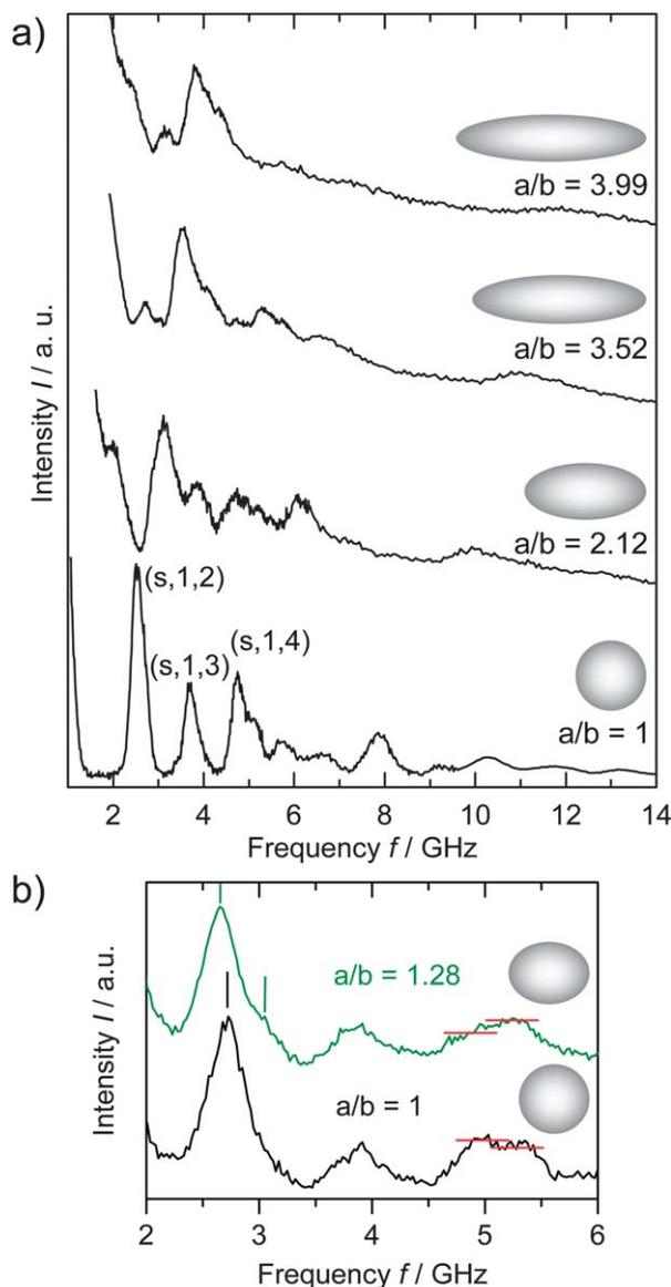
**Fig. 3** (a) Brillouin light scattering (BLS) spectra of the spheroids with three different aspect ratios along with the rich spectrum of the seed spheres displaying the contribution of the principal modes  $(s, 1, l = 2; 3; 4)$  in the low frequency region. (b) Onset of asphericity and the accompanying bifurcation of the lowest frequency  $(s, 1, 2)$  mode due to the lifting of degeneracy in  $m$ .
