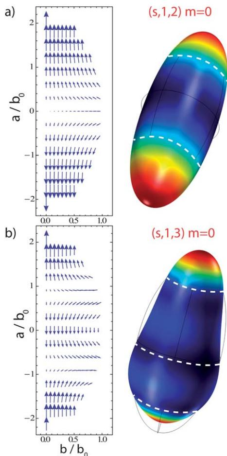
**Fig. 4** Displacement fields of two low frequency modes commonly observed in Brillouin spectroscopy. The depicted aspect ratio corresponds to sample S2, with  $a/b = 2.12$ . (a) First  $m = 0$  mode, mainly derived from  $(s,1,2)$ , with two nodal lines (white dashes) and (b) second  $m = 0$  mode, mainly derived from  $(s,1,3)$ .
