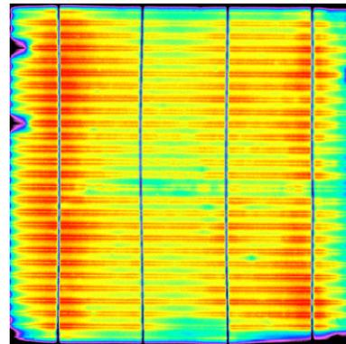
**Figure 6:** Electroluminescence image of a small (5×5 cm<sup>2</sup>) busbar-free solar cell using a flexible foil prototype setup. The wires are running vertically. The image was taken in strong excitation to grant sensitivity towards series resistance effects.
