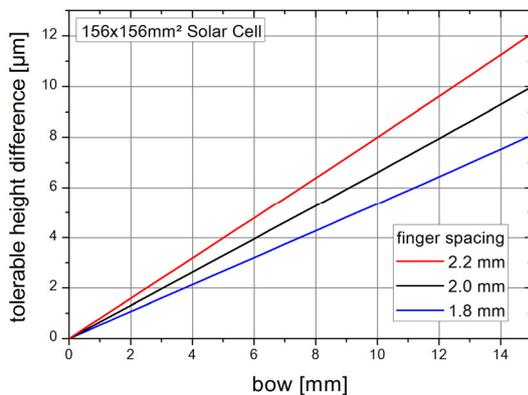
**Figure 4:** Tolerable height difference of the fingers calculated for 156x156 mm<sup>2</sup> solar cells. At differences exceeding the shown value, no proper contact to a lower finger might be achieved.
