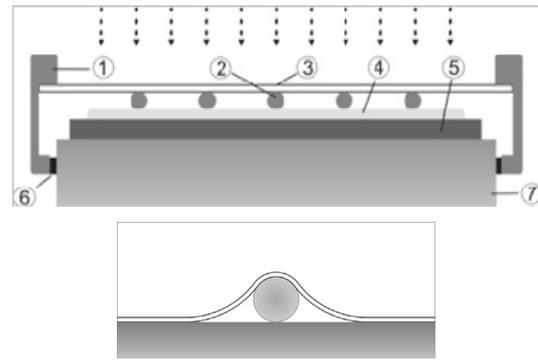
**Figure 5:** (top) Cross-sectional sketch of the setup using wires and a flexible covering foil applied for the electrical characterization of the busbar-free cells. Details: 1 frame, 2 wires, 3 flexible foil, 4 finger, 5 solar cell, 6 airtight seal, 7 chuck; illumination from above. (bottom) The foil is sucked to the cell in between the wires and snuggles to the wires.
