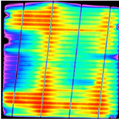
**Figure 7:** Electroluminescence image of a small ( $5 \times 5 \text{ cm}^2$ ) busbar-free solar cell an inelastic plate prototype setup without cavities. The wires are running slightly tilted. The image was taken in strong excitation to grant sensitivity towards series resistance effects. The strong contrast indicates the inhomogeneous pressure on the contact sites.
