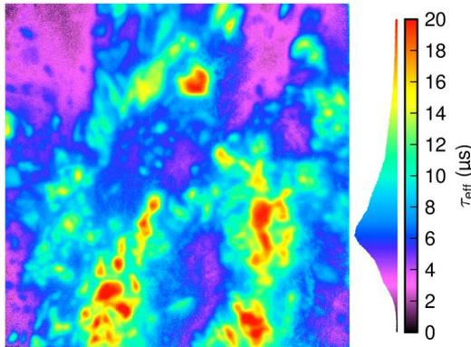
**Figure 4:** TR-PLI lifetime map of a 5 cm wide mc-Si wafer with  $\text{SiN}_x$ -passivation of both surfaces. The illuminating photon flux was  $2.5 \times 10^{17} \text{ cm}^{-2}\text{s}^{-1}$  and the chopper frequency 10 kHz.
