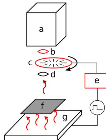
**Figure 1:** Schematic layout of the measurement setup. A Si-wafer (f) is illuminated by the LED panel (g) and emits PL light. The chopper wheel (c) is positioned at the intermediate image plane between the two lenses (b and d) and has a large number of slits. The CCD camera (a) records the chopped PL signal.
