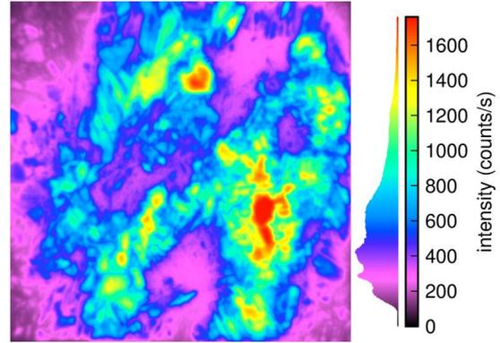
**Figure 5:** Steady-state PL image of the wafer shown in Fig. 4.
