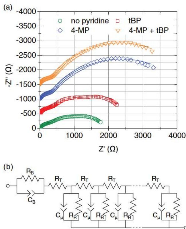
FIG. 2. (a) Nyquist plot of impedance spectra recorded for SQ2 solar cells with different pyridine configurations. Data are acquired at 0 V bias and under white light illumination with approximately  $100 \text{ mW cm}^{-2}$ . Curves are offset in  $500 \Omega$  steps in  $Z'$  direction. Lines represent fit results using the (b) equivalent circuit model for a mesoporous hybrid solar cell (fits are performed with ZView).
