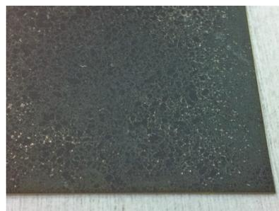
**Figure 1:** Delamination on a FZ sample with a  $\text{SiC}_x/\text{SiN}_x$  stack after a high temperature firing step.
