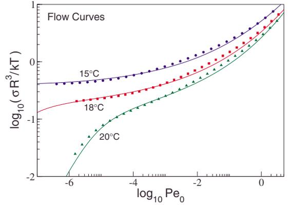
FIG. 12. (Color online) (Experiment) Symbols: the experimentally measured flow curves for three different temperatures,  $T = 20.0$  °C ( $\phi_{\text{eff}} = 0.57$ ),  $T = 18.0$  °C ( $\phi_{\text{eff}} = 0.60$ ), and  $T = 15.0$  °C ( $\phi_{\text{eff}} = 0.65$ ). Lines: theoretical fits to the data using the parameters in Table I.
