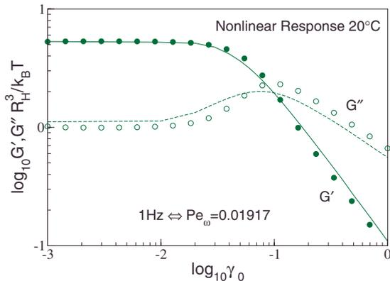
FIG. 16. (Color online) (Experiment) Strain sweeps at a fixed frequency  $Pe_\omega=0.01917$  for the temperature 20 °C. Circles: experimental data. Lines: theoretical predictions.
