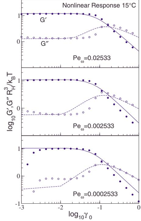
FIG. 14. (Color online) (Experiment) Strain sweeps at three different frequencies for the temperature 15.0 °C. Circles: experimental data. Lines: theoretical fits using the parameter set  $(\epsilon, v_{\sigma}, \Gamma, \gamma_c, \bar{x})$  obtained by simultaneously fitting the flow curves (Fig. 12) and linear-response moduli (Fig. 13).
