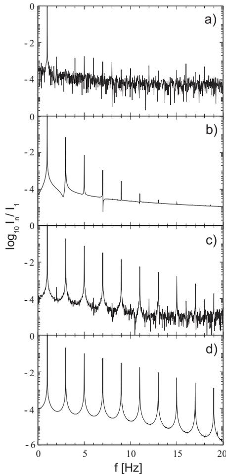
FIG. 19. (Experiment and theory) FFT spectra of the oscillatory time test signals. The experiment was performed at 15.1° and 1 Hz. (a) (experiment) and (b) (theory) are the FFT spectra at  $\gamma_0=0.03$  and (c) (experiment) and (d) (theory) at an amplitude of  $\gamma_0=1$ .
