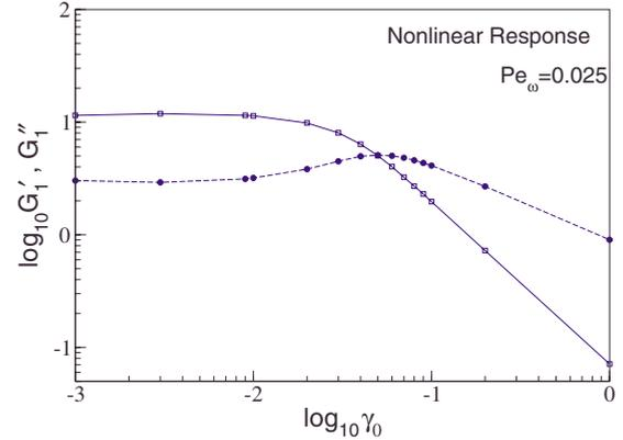
FIG. 9. (Color online) (Simulation) The simulation  $G'_1$  and  $G''_1$  as a function of strain for two-dimensional volume fraction of 0.81 and Peclet number  $\text{Pe}_\omega=0.05$ . For large values of  $\gamma_0$  the moduli obey the power laws  $G''_1 \sim \gamma_0^{-0.68}$  and  $G'_1 \sim \gamma_0^{-1.45}$ .
