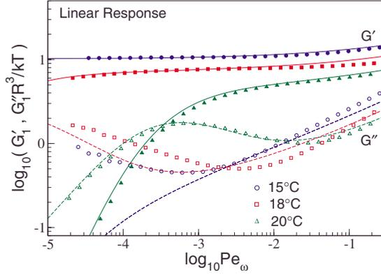
FIG. 13. (Color online) (Experiment) Symbols: the experimentally measured linear-response moduli for three different temperatures,  $T=20.0$  °C ( $\phi_{\text{eff}}=0.57$ ),  $T=18.0$  °C ( $\phi_{\text{eff}}=0.60$ ), and  $T=15.0$  °C ( $\phi_{\text{eff}}=0.65$ ). Lines: theoretical fits to the data using the parameters in Table I.
