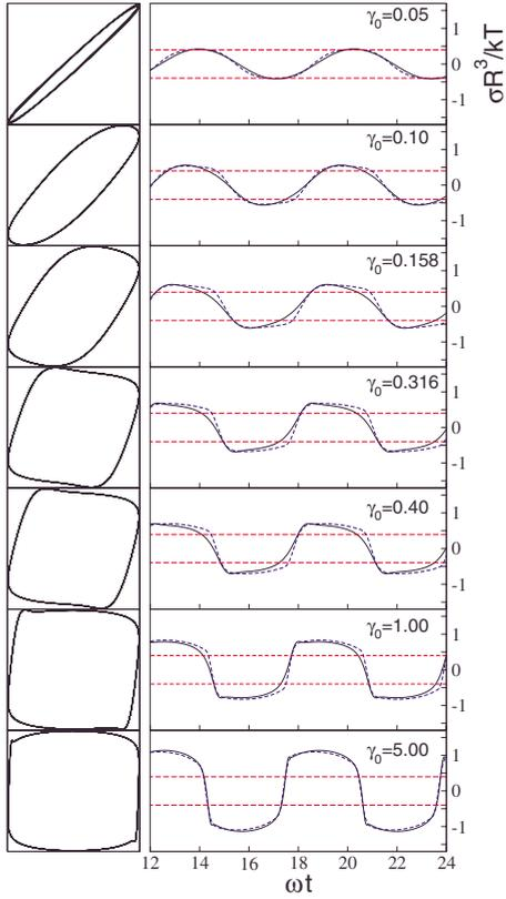
FIG. 18. (Color online) (Experiment) As in Fig. 17 but at a frequency of 0.1 Hz (corresponding to  $Pe_\omega=0.002533$ ). Full black lines: experimental data. Broken blue lines: theoretical results. The yield stress is indicated by the broken red lines.
