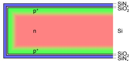
**Figure 1:** Passivated n-type silicon sample with B-emitter,  $\text{SiO}_2$  and  $\text{SiN}_x\text{:H}$  layer.
