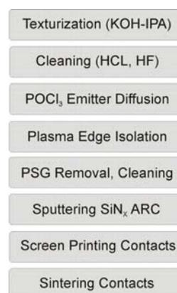
**Figure 1:** Scheme of cell processing steps
