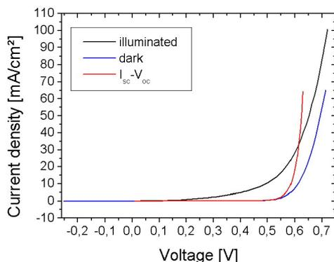
**Figure 1:** Current-voltage measurements of a Cz Si solar cell suffering from a degraded fill factor. The comparison of the  $J_{sc}$ - $V_{oc}$  and the dark  $J(V)$ -curve shows a rather high classical series resistance (splitting up around 0.6V). The illuminated  $J(V)$ -curve (shifted by  $J_{sc}$ ) has a completely different shape responsible for the bad fill factor.
