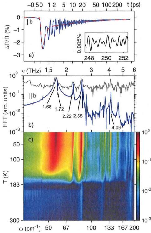
FIG. 1 (color online). (a) Transient change in reflectivity of  $\text{K}_{0.3}\text{MoO}_3$  with  $\vec{E} \parallel \vec{b}$  at 10 K following photoexcitation with a 40 fs laser pulse. Dashed line is the fitted electronic transient. Inset: blowup of the response near 250 ps. (b) The FFT spectrum (amplitude) of the coherent parts of the signals, compared to the recent Raman data (gray) from Ref. [14]. (c) The  $T$  dependence of the corresponding FFT spectrum in the range between 1–6 THz.
