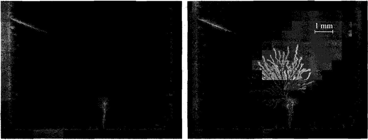
Fig. 7. Magneto-optic images before and after triggering a magnetic instability by an ultrashort laser pulse (half width  $\tau = 150$  fs, energy density  $\approx 10$  mJ/cm<sup>2</sup>,  $\lambda = 819$  nm). The sample was zero field cooled to 10 K before applying a field of  $B_{\text{ext}} = 19.2$  mT.
