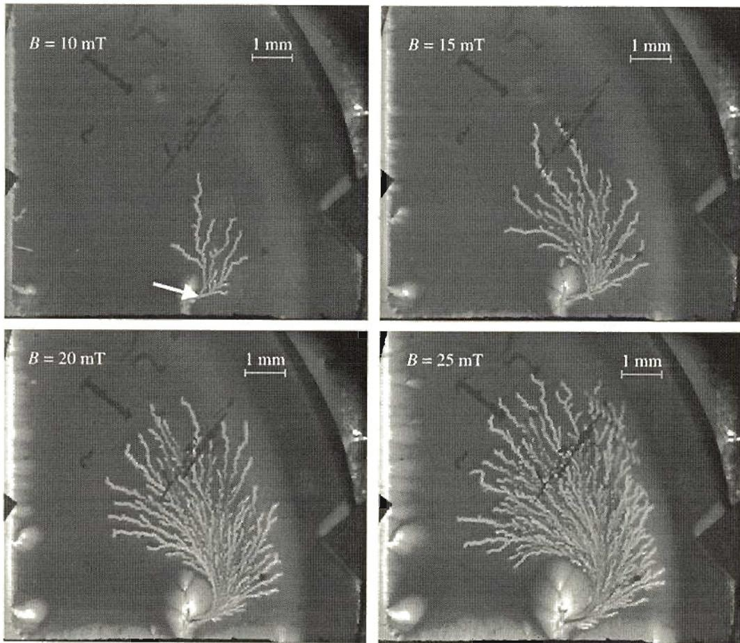
Fig. 6. Magneto-optical images of a YBCO film zero field cooled down to 10 K. The flux distribution after a  $10 \text{ mJ/cm}^2$  laser pulse focused to a  $30 \mu\text{m}$  spot close to the bottom edge of the image (arrow). Above a threshold of  $B_{\text{ext}} = 7.5 \text{ mT}$  the area of the pattern increases linearly with the strength of the external magnetic field applied before the laser pulse.
