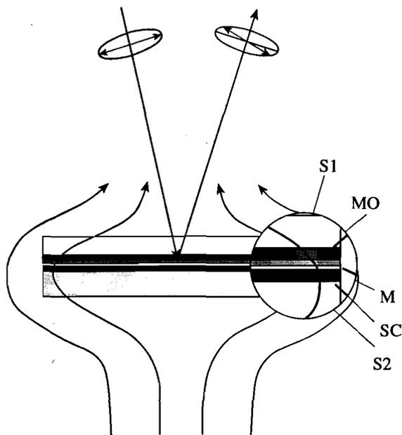
Fig. 1. Schematic drawing of the sample. The incoming light is linearly polarized. S1 = substrate for MO, S2 = substrate for SC, MO = magneto-optically active layer, SC = superconducting sample, M = aluminum mirror.
