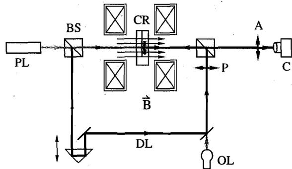
**Fig. 4.** Pump-probe setup used to obtain high time resolution. CR = cryostat with superconducting sample and indicator film, PL = pulse laser, BS = beam splitter, DL = delay line, OL = optional continuous light source, P = polarizer, A = analyzer, C = CCD camera.
