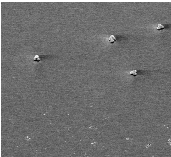
Fig. 4. The edge of a cleaned region after DLC of 800 nm PS spheres. Holes are created at fluences as small as the cleaning threshold laser fluence
