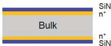
**Figure 2:** Symmetrical sample for  $j_{0e}$  measurement.
