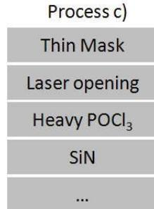
**Figure 4:** Single diffusion selective emitter process
