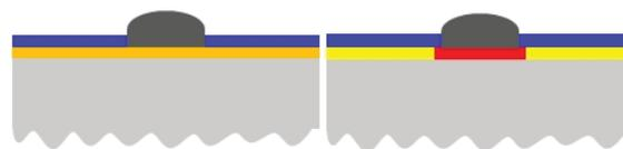
**Figure 1:** Homogeneous (left) and selective (right) emitter.
