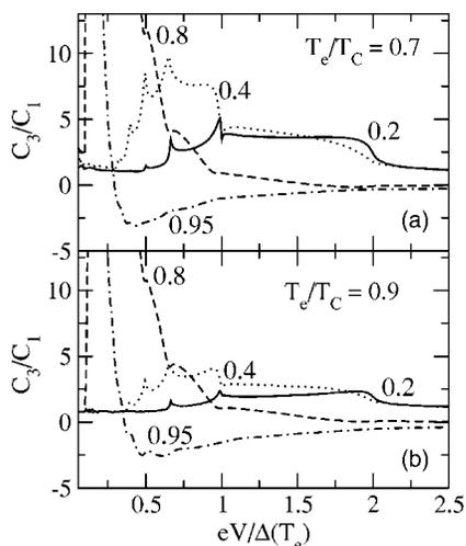
FIG. 14. Ratio  $C_3/C_1$  for two different temperatures as a function of the voltage for a contact between BCS superconductors. The different curves correspond to different transmissions as indicated in the plots.
