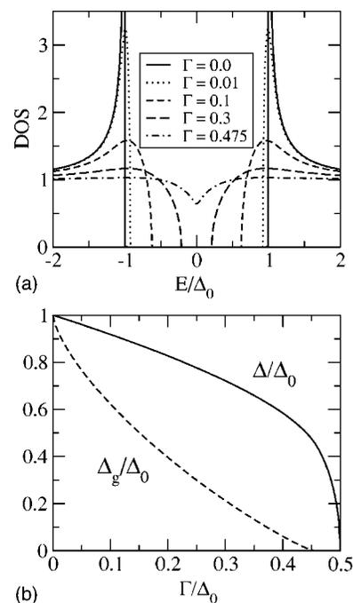
FIG. 4. (a) Density of states as a function of energy of a superconductor for different values of the depairing energy  $\Gamma$  measured in units of gap in the absence of pair-breaking  $\Delta_0$ . (b) Order parameter  $\Delta$  and spectral gap  $\Delta_g$  in units of  $\Delta_0$  as a function of the depairing energy  $\Gamma$  normalized by  $\Delta_0$ .
