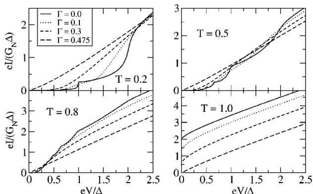
FIG. 5. Zero temperature current-voltage characteristics for superconductors with a depairing energy  $\Gamma$  in units of  $\Delta_0$ . The current and the voltage have been normalized with the order parameter  $\Delta$  at the corresponding  $\Gamma$ . The different panels correspond to different transmissions values.
