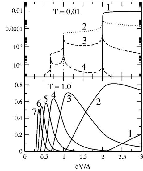
FIG. 3. Average MAR probabilities  $\bar{P}_n(V) \equiv (1/eV) \int_0^{eV} dE P_n(E, V)$  as a function of voltage for a contact between BCS superconductors at zero temperature. The two panels correspond to two different transmissions. The index of the processes is indicated in the plots. Notice the logarithmic scale in the panel (a).
