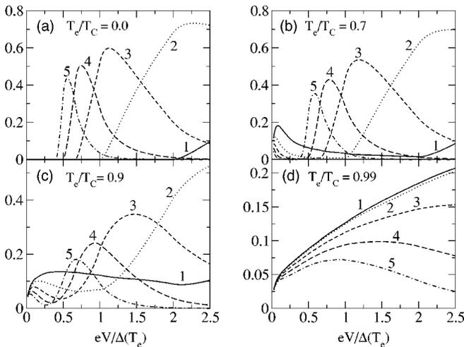
FIG. 13. Average MAR probabilities  $\bar{P}_n(V) \equiv (1/eV) \int_0^{eV} dE P_n(E, V)$  at finite temperature as a function of voltage for a contact between BCS superconductors with transmission  $T=0.95$ . The four panels correspond to different temperatures  $T_e$  expressed in units of the critical temperature  $T_C$ . The index of the processes is indicated in the plots.
