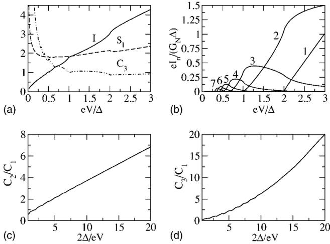
FIG. 9. Zero-temperature transport properties of a short diffusive SNS junction. (a) First three cumulants: current in units of  $(G_N\Delta/e)$ , shot noise in units of  $(2G_N\Delta)$ , and the third cumulant in units of  $(G_N\Delta t_0/hG_0)$ . (b) Current contribution of the different processes. (c) Ratio  $C_2/C_1$  as a function of the inverse of the voltage. (d) Ratio  $C_3/C_1$  as a function of the inverse of the voltage.
