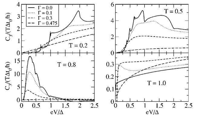
FIG. 8. Zero-temperature third cumulant for superconductors with a depairing energy  $\Gamma$  in units of  $\Delta_0$ . The current and the voltage have been normalized with the order parameter  $\Delta$  at the corresponding  $\Gamma$ . The different panels correspond to different transmissions values.
