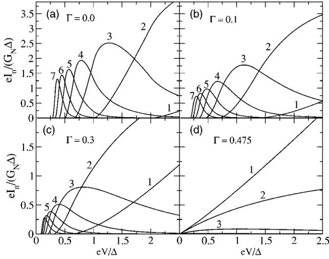
FIG. 6. Current contribution of processes  $n=1, 2, \dots$  for  $T=1$  as a function of voltage for superconductors with a depairing energy  $\Gamma$  in units of  $\Delta_0$ . The current and the voltage have been normalized with the order parameter  $\Delta$  at the corresponding  $\Gamma$ . The order of the processes is indicated in the plots.
