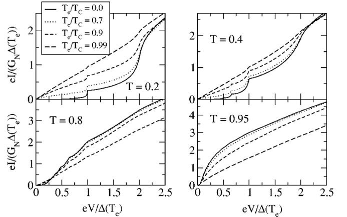
FIG. 10. Current-voltage characteristics at finite temperature for BCS superconductors. The temperature is in units of the critical temperature  $T_C$ . The current and the voltage are normalized with the temperature-dependent gap. The different panels correspond to different transmission values.
