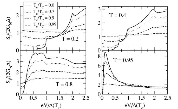
FIG. 11. Finite temperature noise for BCS superconductors. The temperature is normalized with the critical temperature  $T_C$ . The different panels correspond to different transmission values. The voltage is normalized with the temperature-dependent gap, and the current with the zero-temperature gap. Note that the scaling is different from the other plots in this section.
