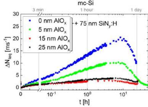
**Figure 4:** Time-dependent lifetime equivalent defect density of mc-Si samples, passivated with  $\text{AlO}_x$  of different thickness and subsequent 75 nm  $\text{SiN}_y\text{:H}$  after firing. Data calculated with extracted PCD lifetimes at elevated temperature at  $\Delta n = 0.1 \times p_0$ . As the 0 nm  $\text{AlO}_x$  sample (processed as standard) broke during characterization, the 0 nm  $\text{AlO}_x$  sample with additional time adjustment is shown here.
