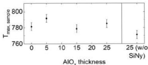
**Figure 6:** Measured sample peak temperatures during fast firing plotted against the AlO<sub>x</sub> thickness within the AlO<sub>x</sub>/SiN<sub>y</sub>:H layer system. Set peak temperature of the belt furnace was 800°C.
