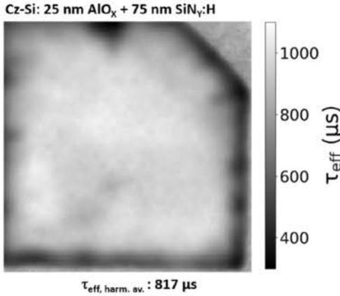
**Figure 3:** TR-PLI lifetime map at room temperature of a Cz-Si sample deposited with 25 nm  $\text{AlO}_x$  and 75 nm  $\text{SiN}_y\text{:H}$  shows a homogeneous passivation quality.
