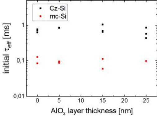
**Figure 2:** Initial  $\tau_{\text{eff}}$  measured by PCD at room temperature and extracted at  $\Delta n = 0.1 \times p_0$  of all mc-Si and Cz-Si samples with different  $\text{AlO}_x$  layers (0-25 nm) and subsequent  $\text{SiN}_y\text{:H}$  passivation.
