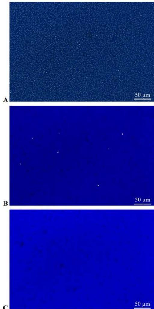
**Figure 3:** Optical microscopy images after firing step of  $AlO_x/SiN_y:H$  stacks deposited using ALD (A), APCVD at 700°C set (B) and APCVD at 590°C set (C) for  $AlO_x$  deposition. Blistering is only visible in (A), pin holes are seen in (A) and (B).
