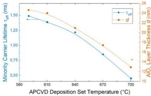
**Figure 2:**  $\tau_{eff}$  (left axis) and layer thickness (right axis) dependent on the APCVD deposition set temperature.
