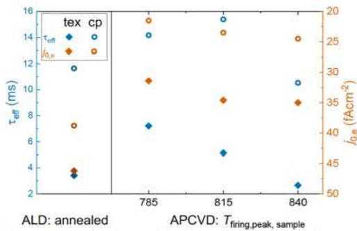
**Figure 4:** Passivation quality determined by measuring  $\tau_{\text{eff}}$  for undiffused samples (left axis, blue symbols) and by measuring  $j_{0,e}$  for samples with a  $65 \text{ } \Omega/\text{sq}$   $p^+$  emitter (right axis, orange symbols). Annealed ALD  $\text{AlO}_x$  reference in the left part of the graph, at a variety of temperatures fired APCVD  $\text{AlO}_x/\text{SiN}_y\text{:H}$  stacks reference in the right part of the graph.
