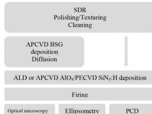
**Figure 1:** Schematic process flow of samples shown in the results section.
