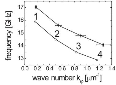
FIG. 3. The frequencies of the four highest modes as a function of their wave numbers at  $\mu_0 H_{\text{bias}} = 80$  mT obtained by experiment (solid dots) and by simulation (open circles). The lines are guides to the eye. The numbers label the different modes.
