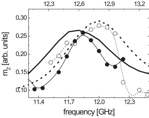
FIG. 5. The global Fourier transform of simulated (lines) data together with experimental data from frequency sweeps using SR-FMR-MOKE (dots and lines) for the remanent onion state at  $\mu_0 H_{\text{bias}} = 0$  mT. Simulated and experimental data correspond to the lower and upper frequency axis, respectively. The solid and the dashed lines represent the single and the coupled ring, respectively.
