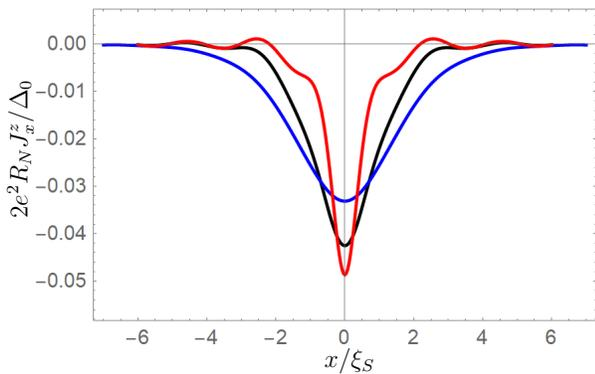
FIG. 5. Spin current  $J_x^z(x)$  at the plane DW in equilibrium. Other components of the spin current are zero.  $l_{DW} = \xi_S$  (blue);  $0.5\xi_S$  (black);  $0.2\xi_S$  (red).  $\xi_S = v_F/\Delta_0$  throughout the paper.  $h_{eff} = 0.3\Delta_0$ ,  $T = 0.02\Delta_0$ .
