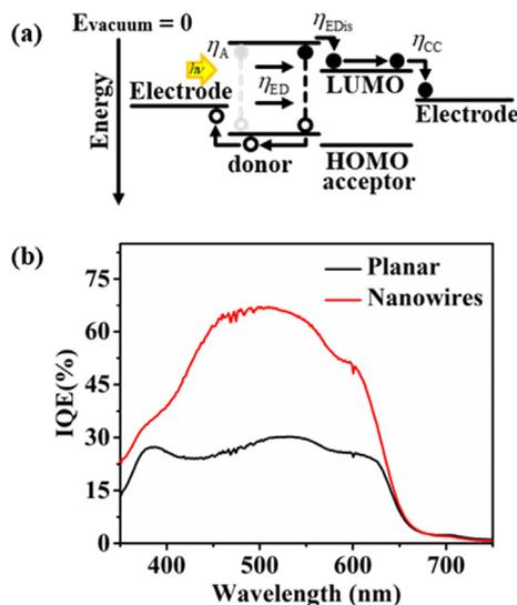
Fig. 2. (a) Schematic diagram of the working principles of typical organic solar cells, where  $\eta_A$  is the absorption efficiency,  $\eta_{ED}$  is the exciton diffusion efficiency,  $\eta_{EDis}$  is the exciton dissociation efficiency, and  $\eta_{CC}$  is the charge collection efficiency. (b) Internal quantum efficiency (IQE) for the non-transparent planar (black) and Ag/ZnO core-shell nanowire (red) solar cells, under short circuit condition without background illumination.
