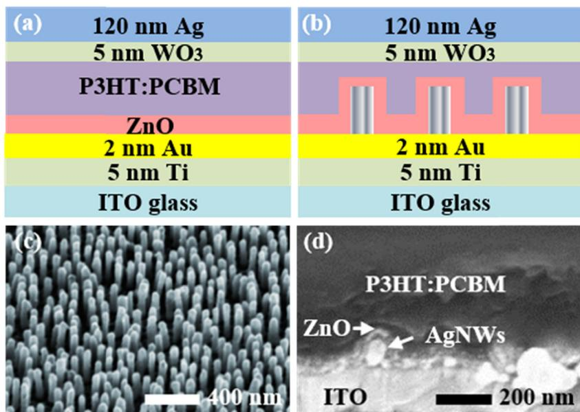
Fig. 1. (a–b) Schematic illustrations of the non-transparent planar and Ag/ZnO core-shell nanowire organic solar cells, respectively. (c) Typical scanning electron spectroscopy (SEM) side view of the free-standing silver nanowire arrays at a stage degree of 54°. (d) A cross-sectional SEM image of the Ag/ZnO core-shell nanowire organic solar cells without the top electrodes at a stage degree of 54°.
