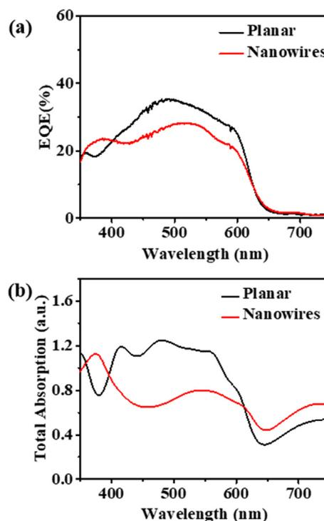
Fig. 3. (a) External quantum efficiency (EQE) for the non-transparent planar (black) and Ag/ZnO core-shell nanowire (red) organic solar cells, under short circuit condition without background illumination. (b) Total absorption spectra for the non-transparent planar (black) and Ag/ZnO core-shell nanowire (red) organic solar cells.
