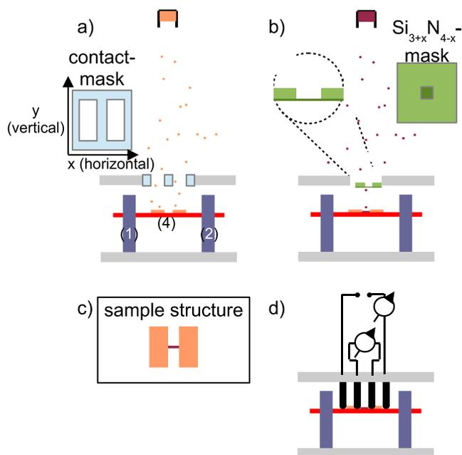
FIG. 1. (Color online) Principle of the modular holder system for which all preparations can be performed in UHV. The sample (4) is attached via posts (1,2) to the sample holder. (a) First mask holder for evaporation of macroscopic contact pads (contact mask). (b) Second mask consisting of a nanostructured  $\text{Si}_{3+x}\text{N}_{4-x}$  membrane. (c) Schematic of the ideal nanoscale bridge structure. (d) Four-point contact for *in situ* electronic measurements.
