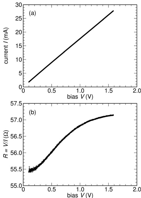
FIG. 4. (a) Measurement of the current as a function of voltage of a Au sample contacted by the method described above. (b) Calculated resistance as a function of voltage from the measurement shown in (a).
