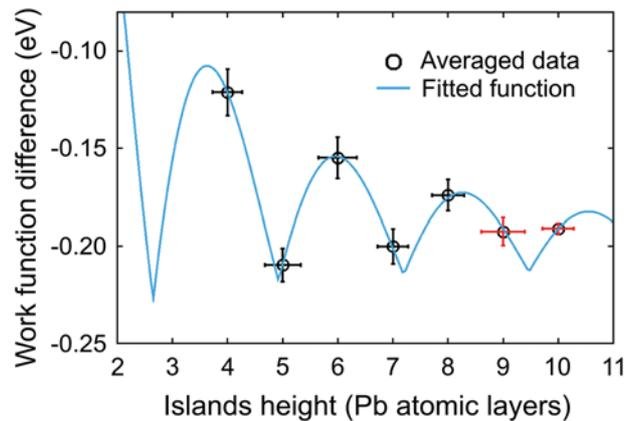
Fig. 4 Quantum oscillations in the local work function of ultra-thin Pb islands on Si(111) as a function of the island height measured from the WL obtained with SFM/KPFM. The LWF exhibits a damped even-odd oscillation with increasing island height. The two points with red error bars result from a small number of data. Data fitted with eqn (6).
