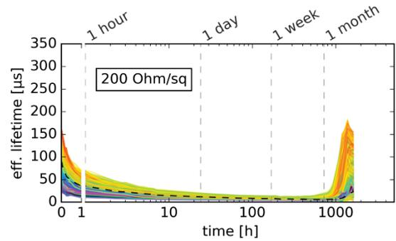
**Figure 4:** Effective lifetimes for a sample with emitter sheet resistivity of 200  $\Omega/\text{sq}$  (x-axis: 0-1 h linear scale, 1-2000 h log scale).
