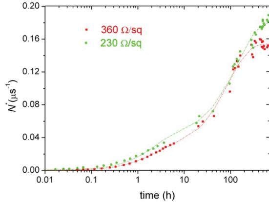
**Figure 5:** Evolution of  $N^*$  for the samples with  $R_{\text{sheet}}$  of 230 and 360  $\Omega/\text{sq}$ . The solid lines are numerically simulated by solving Eq. (2) using the coefficients from Tab. I.
