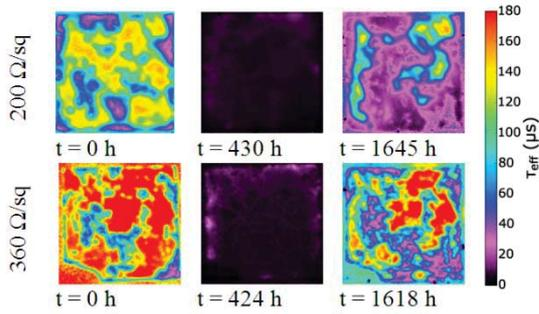
**Figure 2:** Effective lifetime mappings for samples with  $R_{\text{sheet}}$  of 200  $\Omega/\text{sq}$  (upper row) and 360  $\Omega/\text{sq}$  (lower row) directly after firing (left), around maximum degradation (middle) and after onset of regeneration (right).
