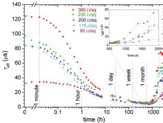
**Figure 3:** Evolution of the average  $\tau_{\text{eff}}$  for the samples with different emitter layers (75°C, 0.9 suns).
