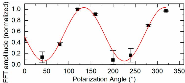
**Figure 3.** Peak amplitude value of the response of the LiNbO<sub>3</sub> layer plotted as a function of the polarization angle of the incident pulse. The red solid line shows a fit through the experimental data points (black squares) which exhibits a sinusoidal behaviour with  $\pi$  periodicity. The error is estimated by the mean average of the noise floor together with the standard deviation.
