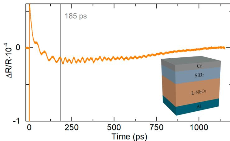
**Figure 1.** Transient reflectivity changes of the sample. Inset: Sample structure; from top to bottom, the sample consists of a layer of 18-nm Cr, 1140-nm SiO<sub>2</sub>, 325- $\mu$ m LiNbO<sub>3</sub>, and 100-nm Al (thicknesses are not to scale).
