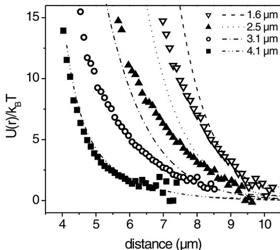
FIG. 3. Experimentally determined interaction energy  $U(r)$  (symbols) for two particles in a line tweezers in the presence of a fixed third particle with distance  $d$  on the perpendicular bisector of the line trap. For comparison the superposition of three pair potentials is plotted as lines. Symbols and lines are labeled by the value of  $d$ .
