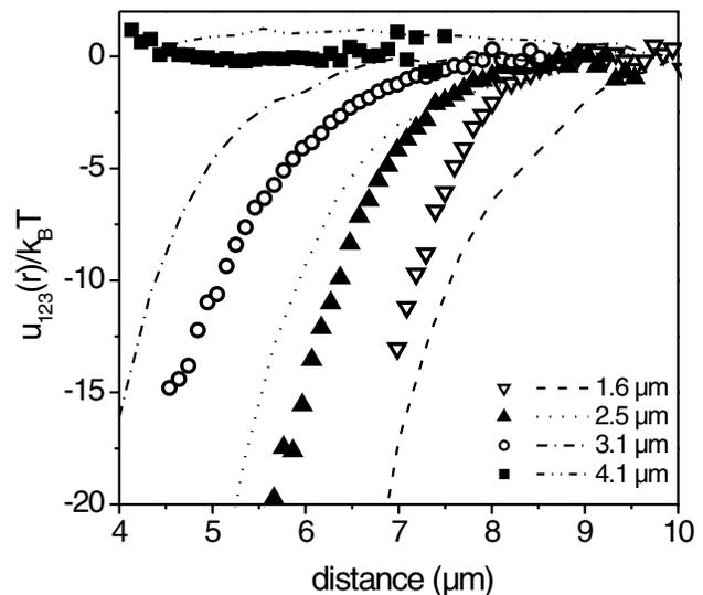
FIG. 4. Three-body potentials for different  $d$ . Measured three-body potentials are indicated by symbols. The lines are three-body potentials as obtained from the solution of the nonlinear Poisson-Boltzmann equation for three colloids arranged as in the experiment. The parameters in the Poisson-Boltzmann calculation were chosen such that the pair-interaction potentials were correctly reproduced. Symbols and lines are labeled by the value of  $d$ .
