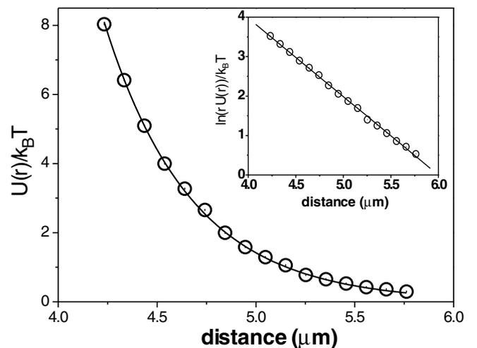
FIG. 2. Measured pair-interaction potentials (symbols) in the absence of the third particle. The data agree well with a Yukawa potential (solid line). In the inset the potential is multiplied by  $r$  and plotted logarithmically, so that Eq. (1) transforms into a straight line.
