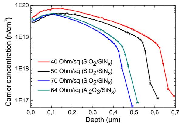
Fig. 2. Doping profiles of the PECVD B emitters measured by an electrochemical capacitance voltage setup.
