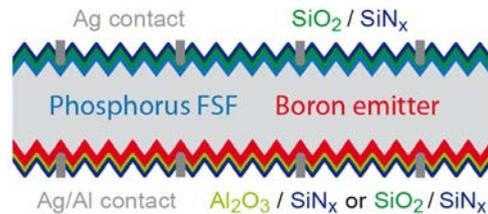
Fig. 1. Cross-section: n-type bi-facial solar cell with PECVD B emitter and P FSF. Contact formation is conducted via screen-printing of Ag paste on P FSF and Ag/Al paste on the B emitter. Two different passivation layer stacks ( $\text{Al}_2\text{O}_3/\text{SiN}_x$  and  $\text{SiO}_2/\text{SiN}_x$ ) are used for emitter passivation.
