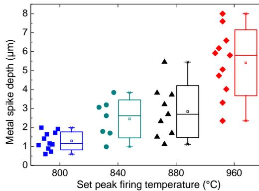
Fig. 6. Depths of the metal spikes determined by SEM images of FIB cross sections of the contact spots.
