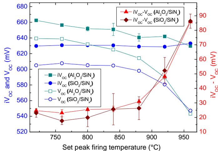
Fig. 4. Evolution of  $V_{OC}$  and implied  $V_{OC}$  as well as the difference  $iV_{OC} - V_{OC}$ , which is attributed to the metal induced losses. The metal induced losses are strongly increasing with increasing set peak firing temperatures and independent of the passivation layer stack.
