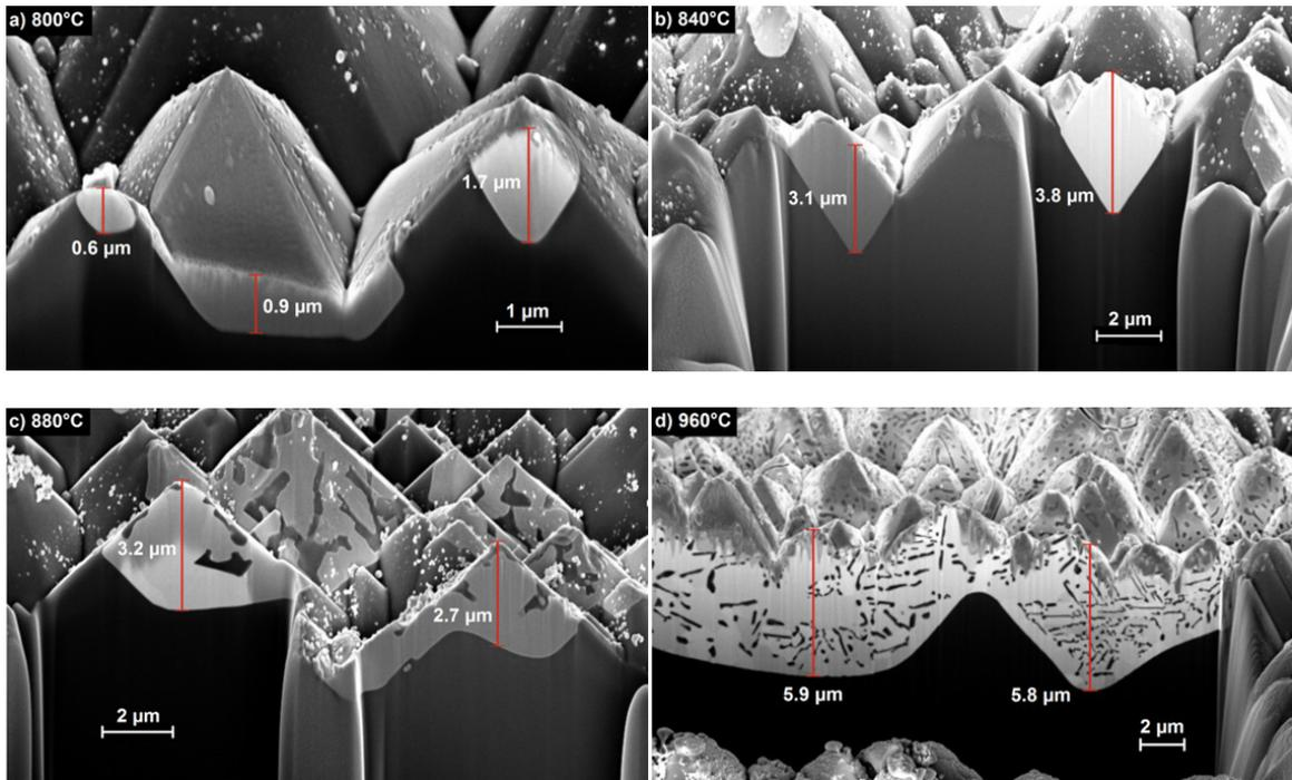
Fig. 5. SEM images of FIB cross sections of the contact spots for different SPFT (given in the upper left corners). The depths of the Ag/Al spikes are marked with red lines. Area density and average depth of the spikes are increasing strongly with increasing SPFT.
