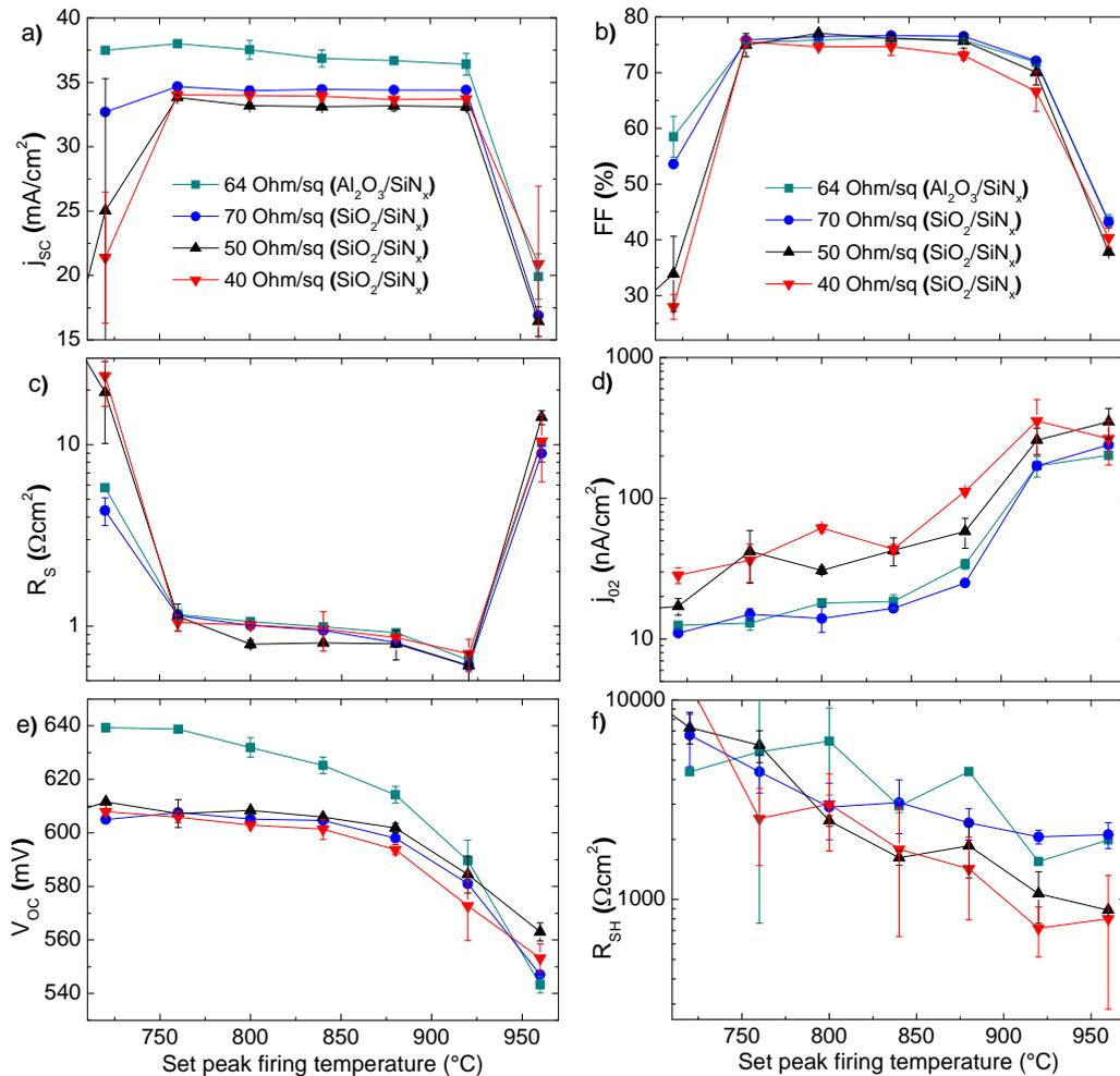
Fig. 3. IV-characteristics of the bi-facial solar cells measured with a h.a.l.m. flasher.
