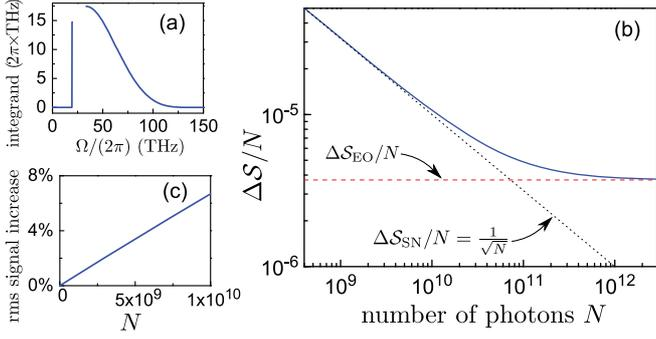
FIG. 2 (color online). (a) Calculated integrand function  $\Omega/(n/n_\Omega)|R(\Omega)|^2$  entering Eq. (13). (b) Double logarithmic plot of the ratio  $\Delta S/N$  in dependence on  $N$ . The black dotted (red dashed) line shows the bare SN (multi THz vacuum) contribution. (c) Increase of  $(\Delta S - \Delta S_{SN})/\Delta S_{SN}$  with  $N$ . Parameters are defined in the main text.
