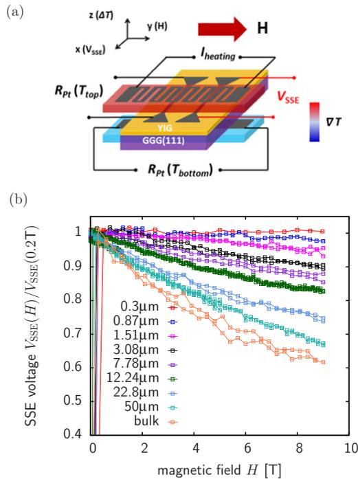
FIG. 3. (Color online) (a) Schematic diagram of sample structure and measurement setup. (b) Normalized spin Seebeck voltage  $V_{\text{SSE}}(H)/V_{\text{SSE}}(0.2 \text{ T})$  of Pt/YIG structures composed of YIG single crystal and selected YIG thin films with thickness ranging from 0.3 to  $50 \mu\text{m}$ .
