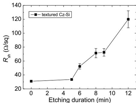
Fig. 2.  $R_{sh}$  of a 30  $\Omega/sq$  B doped layer (as-diffused) on a textured Cz-Si surface versus B-EEB duration. The error bars result from the variation of  $R_{sh}$  determined in different locations on the 125×125 mm<sup>2</sup> wafer by four-point probe method.
