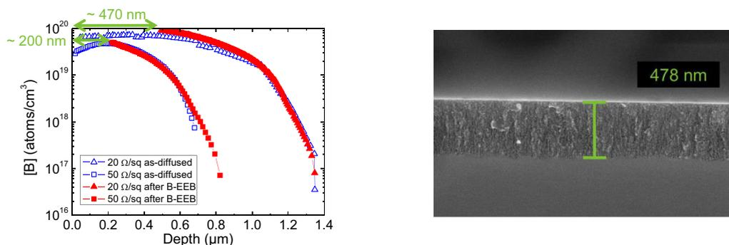
Fig. 1. Left: B concentration profile of a 20 and 50  $\Omega/\text{sq}$   $\text{p}^+$  region after  $\text{BBr}_3$  diffusion and after subsequent B-EEB to 100  $\Omega/\text{sq}$  determined by ECV. Right: Cross sectional SEM micrograph of the 20  $\Omega/\text{sq}$   $\text{BBr}_3$  diffused Si wafer surface etched-back to 100  $\Omega/\text{sq}$  by creating a  $\sim 470 \text{ nm}$  thick por-Si layer.
