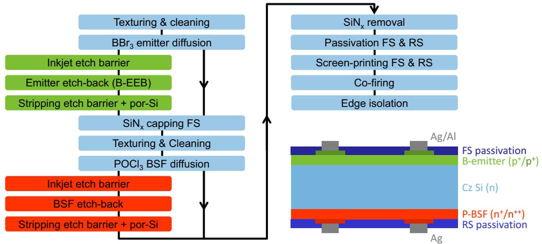
Fig. 4. Processing sequence for screen-printed bifacial n-type solar cells with optional steps for selective p<sup>+</sup> emitter and selective n<sup>+</sup> BSF; schematic representation of the final solar cell featuring selective doping structures on both sides.
