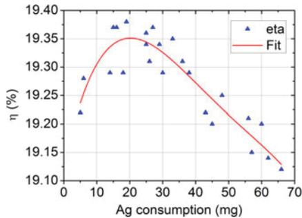
Fig. 6. The efficiency plotted versus the LIP Ag consumption for solar cells with an Ag plated front grid.
