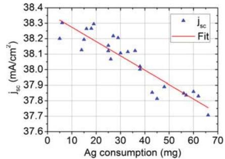
Fig. 4. Current density plotted versus the Ag consumption for solar cells with an Ag plated front grid. A reduction of Ag leads to higher current densities of the device because of reduced shading.
