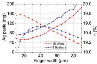
Fig. 2. Ag paste consumption (solid lines) and efficiency (dashed lines) plotted versus the finger width of screen printed solar cells.
