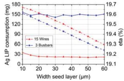
Fig. 3. Optimal amount of plated Ag needed plotted versus the seed layer width (solid lines). Efficiencies of both cell types (dashed lines).
