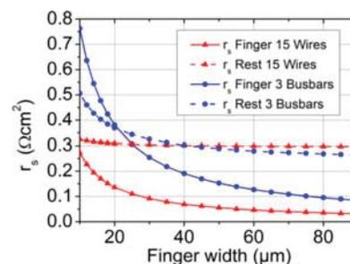
Fig. 1. Series resistance contribution plotted versus the width of a screen printed finger of a multi-busbar and a three-busbar solar cell. In the dashed lines, the remaining part of the series resistance is plotted. By adding the finger contribution to the rest, one obtains the total series resistance of the solar cells.
