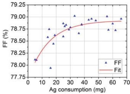
Fig. 5. Fill factor plotted versus the Ag consumption for solar cells with an Ag plated front grid. For a sufficient fill factor, the amount of Ag has to be adapted.
