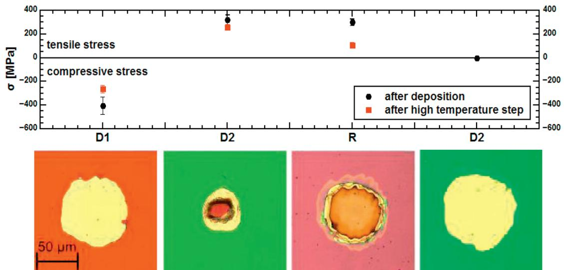
Fig. 4. Intrinsic stress  $\sigma$  and respective microscopy pictures after single laser pulse treatment for all silicon nitride layers D1, D2 and R. Changing the PECVD deposition parameters for D2 leads to a stress-free dielectric layer (far right)
