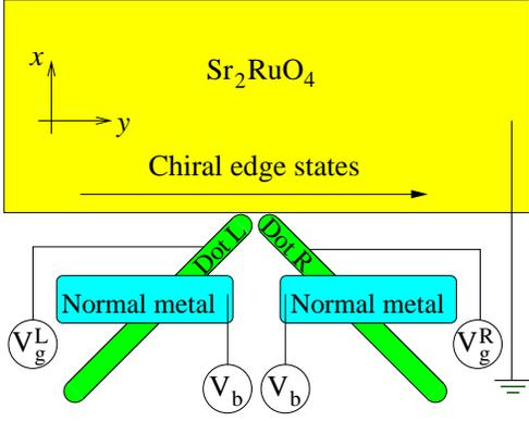
FIG. 1: Schematic of the device (not to scale). Two single-walled carbon nanotubes (or one bent nanotube) are used to form a double-dot system tunnel-coupled to a thin platelet of  $\text{Sr}_2\text{RuO}_4$ .
