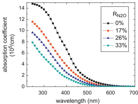
Fig. 2. Spectral absorption coefficient  $\alpha$  of a-SiO<sub>x</sub>N<sub>y</sub>:H films deposited at various N<sub>2</sub>O dilutions ( $T_{dep}=175$  °C,  $P=100$  W).
