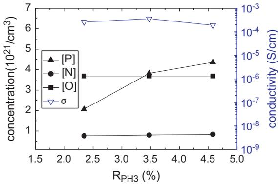
**Fig. 8.** Phosphorus, nitrogen and oxygen concentration (left axis) and dark conductivity (right axis) of (n) a-SiO<sub>x</sub>N<sub>y</sub>:H films as a function of PH<sub>3</sub> dilution. ( $T_{dep}=300$  °C,  $R_{N_2O}=16.5\%$ , and  $P=20$  W).
