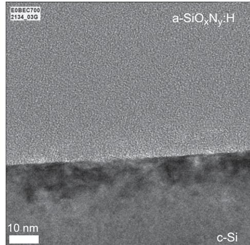
**Fig. 4.** HRTEM image of an intrinsic a-SiO<sub>x</sub>N<sub>y</sub>:H film on a c-Si substrate. Neither clusters nor nanoparticles are visible within the a-SiO<sub>x</sub>N<sub>y</sub>:H film. The dark regions in the c-Si close to the interface might be strains due to plasma damage.
