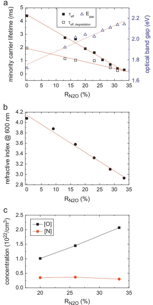
**Fig. 1.** (a) Effective minority carrier lifetime and optical band gap, (b) refractive index (real part)  $n$ , and (c) oxygen and nitrogen concentration of a-SiO<sub>x</sub>N<sub>y</sub>:H films as a function of N<sub>2</sub>O dilution in silane ( $T_{dep}$ =175 °C,  $P$ =100 W).
