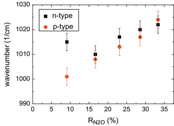
**Fig. 9.** Peak position of Si–O–Si stretching mode vibrations of phosphorus- (black squares) and boron- doped (red diamonds) a-SiO<sub>x</sub>N<sub>y</sub>:H films as a function of N<sub>2</sub>O dilution determined by means of FTIR measurements ( $T_{dep}=300$  °C,  $R_{B_2H_6}/PH_3=2.3\%$ , and  $P=5$  or 20 W). (For interpretation of the references to color in this figure legend, the reader is referred to the web version of this article).
