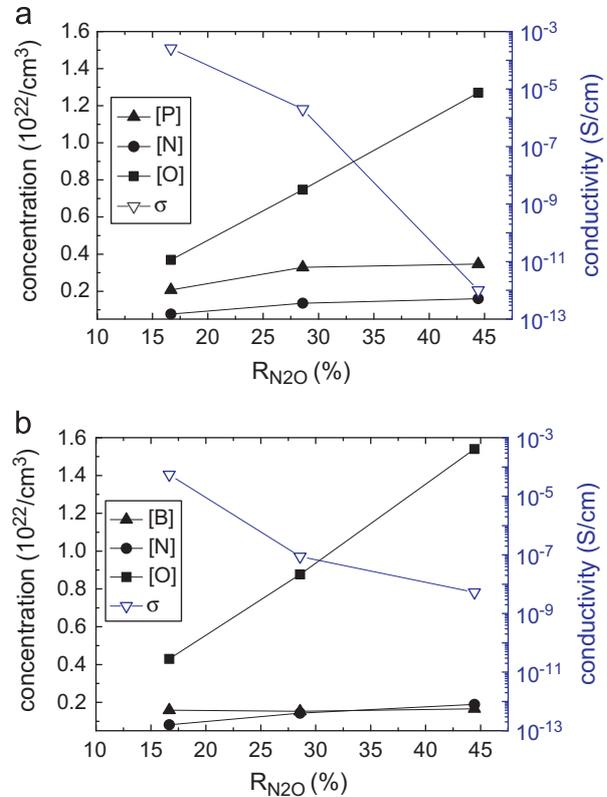
**Fig. 7.** Phosphorus/boron, nitrogen and oxygen concentration (left axis) and dark conductivity (right axis) of (a) (n) a-SiO<sub>x</sub>N<sub>y</sub>:H films and (b) (p) a-SiO<sub>x</sub>N<sub>y</sub>:H films as a function of N<sub>2</sub>O dilution ( $T_{dep}=300$  °C,  $R_{PH_3}=R_{B_2H_6}=2.3\%$ ,  $P_{PH_3}=20$  W, and  $P_{B_2H_6}=5$  W).
