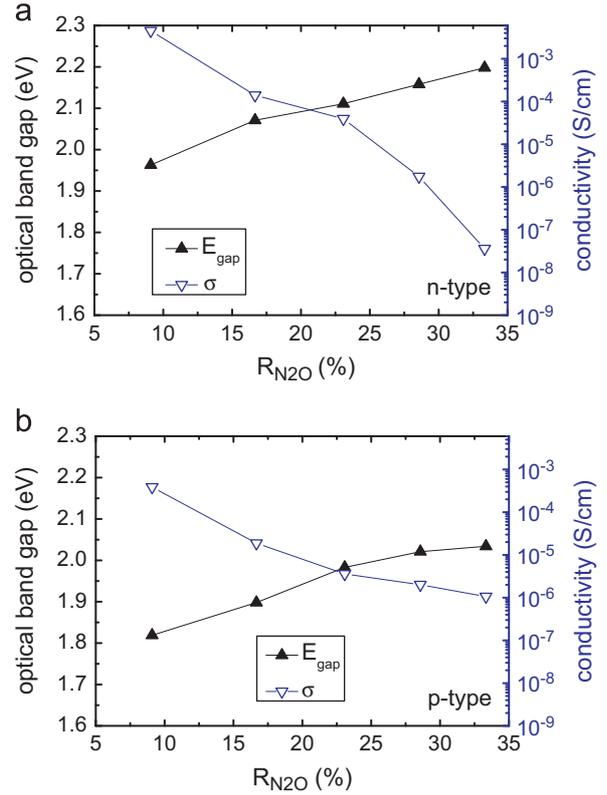
**Fig. 6.** (a) Optical band gap (left axis) and dark conductivity (right axis) of (n) a-SiO<sub>x</sub>N<sub>y</sub>:H films and (b) (p) a-SiO<sub>x</sub>N<sub>y</sub>:H films as a function of N<sub>2</sub>O dilution ( $T_{dep}=300$  °C,  $R_{PH_3}=R_{B_2H_6}=2.3\%$ ,  $P_{PH_3}=20$  W, and  $P_{B_2H_6}=5$  W).
