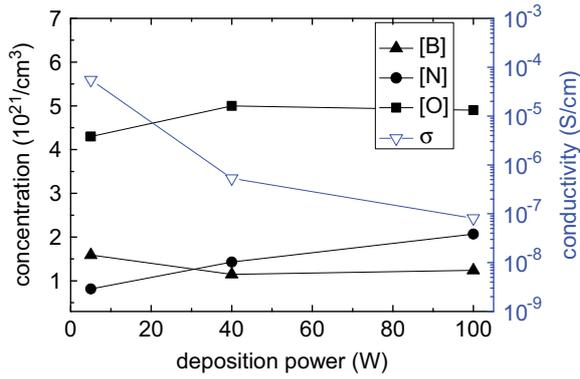
**Fig. 5.** Boron, nitrogen and oxygen concentration (left axis) and dark conductivity (right axis) of (p) a-SiO<sub>x</sub>N<sub>y</sub>:H films as a function of deposition power ( $T_{dep}=300$  °C,  $R_{N_2O}=16.5\%$ ,  $R_{B_2H_6}=2.3\%$ ).
