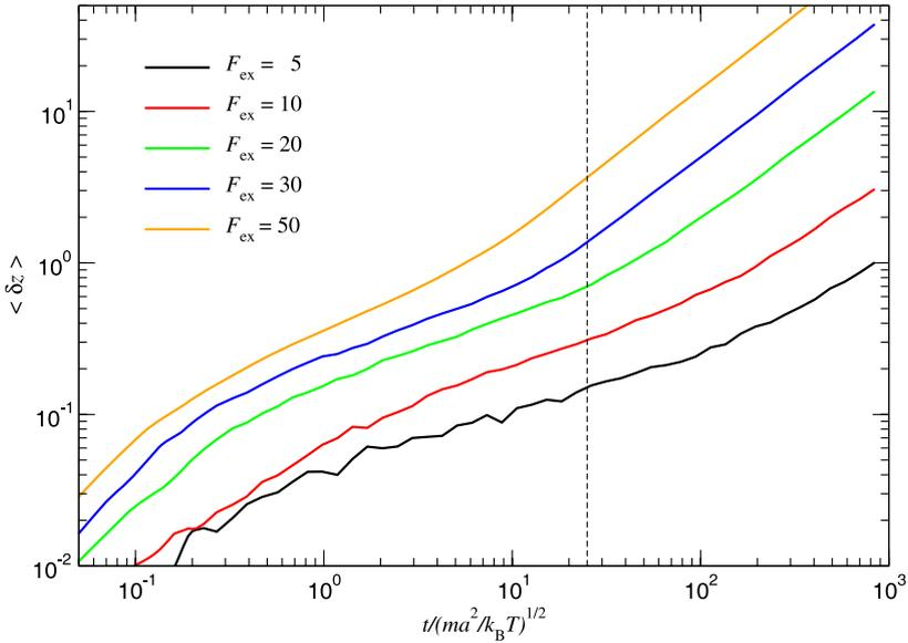
**Fig. 6.** Linear displacement of the forced tracer particle in direction of the force (given in  $k_B T/a$ ) for the density  $\varphi = 0.57$  from Langevin dynamics simulations. The intermediate time  $t = 25\sqrt{ma^2/k_B T}$  at which probe-particle distributions were sampled is indicated by the dashed vertical line.
