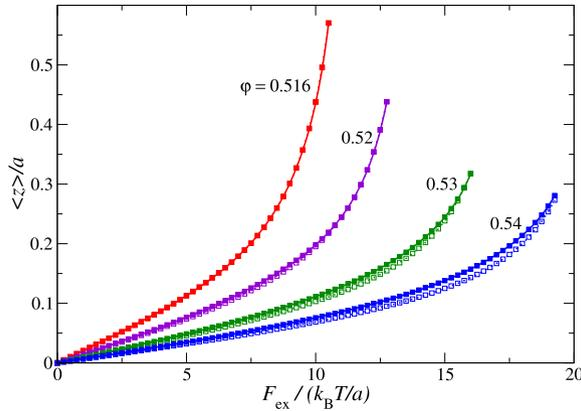
**Fig. 3.** Mean value  $\langle z \rangle$  of the long-time limit of the probe-particle displacement along the force direction as function of the external force  $F_{ex}$ . Curves for different glass packing fractions  $\phi$  are shown as labeled. At the higher two  $\phi$ , corrected (filled squares) and uncorrected (open squares)  $\langle z \rangle$  differ slightly; see text for details.
