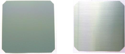
**Figure 2:** Photograph of 156×156 mm<sup>2</sup> pseudo-square monocrystalline silicon wafers sawn with a slurry process (left) and a diamond wire process (right).
