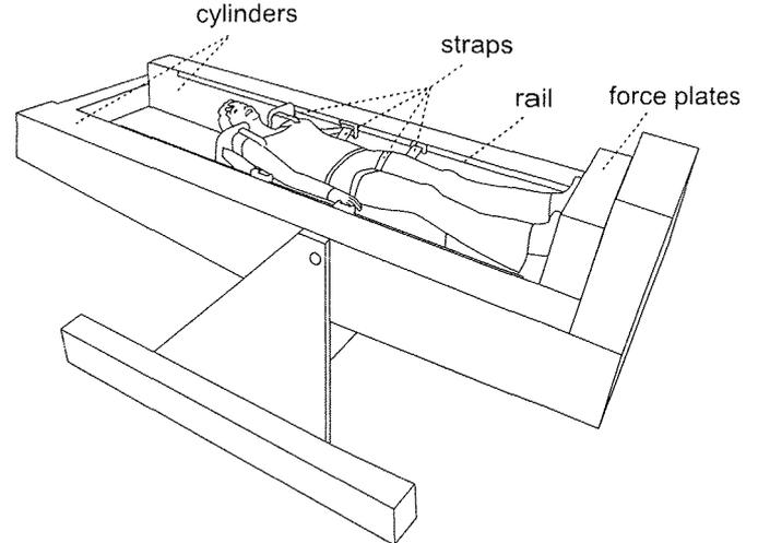
**Fig. 1.** Sledge jump system in the horizontal position. The participant is fixed to the wooden sledge with straps. The straps are attached to the rails and can slide in the direction of the rails. The participant stands on two force plates (separated, one for each foot). Reprinted from Kramer et al., (2010), with permission from Elsevier.
