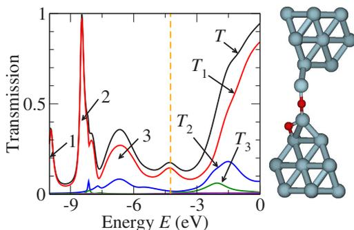
FIG. 9. (Color online) Al-O<sub>2</sub>-Al: Example of a possible geometrical configuration when the Al tip atoms are included in the relaxation process in addition to the molecule, and the corresponding transmission as a function of energy. The vertical dashed line indicates the Fermi energy.
