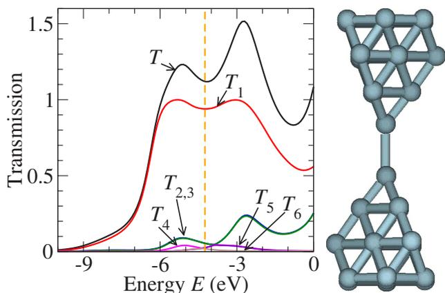
FIG. 3. (Color online) Al-Al: Transmission as a function of energy. Both the total transmission ( $T$ ) and its channel contributions ( $T_n$ ) are shown. The vertical dashed line indicates the Fermi energy of bulk Al. The corresponding contact geometry with a distance of 3.4 Å between the Al tip atoms is depicted on the right.
