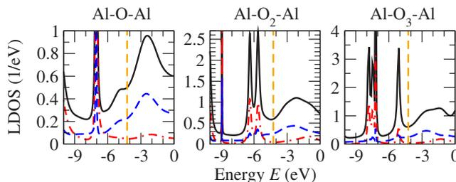
FIG. 5. (Color online) Al-O<sub>x</sub>-Al: LDOS corresponding to the second row in Fig. 4. The solid (black) curve is for the region including the Al tip atoms and the O atoms, the dash-dotted (red) one is for one of the oxygen atoms, and the dashed (blue) curve is for one of the Al tip atoms. The vertical dashed (orange) line indicates the Fermi energy.
