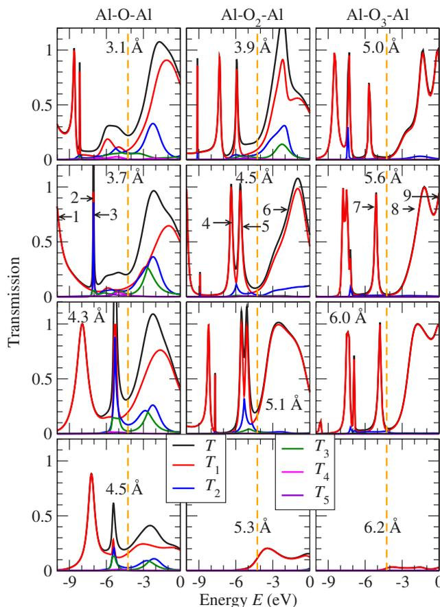
FIG. 4. (Color online) Al-O<sub>x</sub>-Al: Transmission as a function of energy for the structures shown in Fig. 1. The tip-to-tip distance increases from the top to the bottom and is given in the panels. The vertical dashed lines indicate the Fermi energy.
