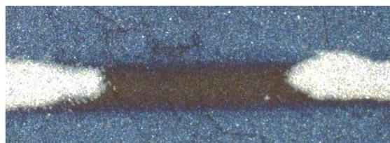
**Figure 4:** Partly removed etching paste after several seconds in the ultrasonic bath. The removal had to be optimized due to the isotropic textured surface condition.
