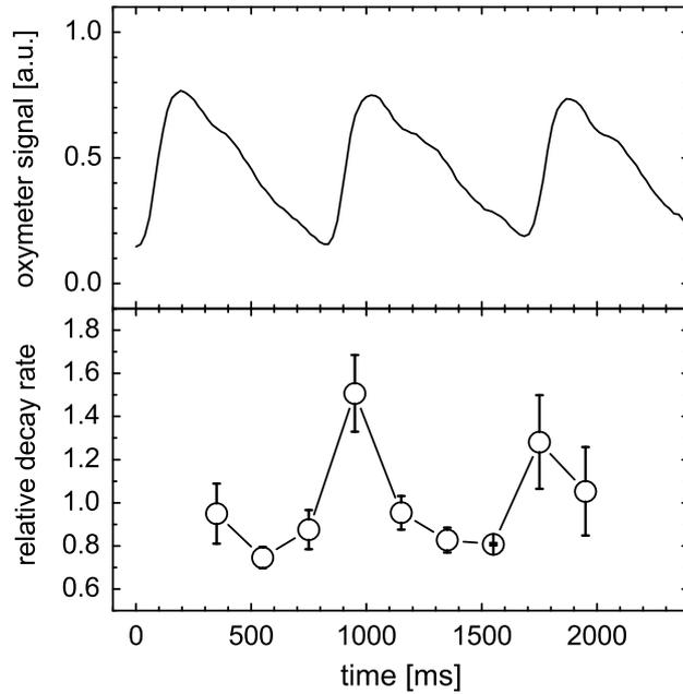
Fig. 7. Oxymeter signal recorded at the ring finger tip (top) and relative decay rate of the intensity autocorrelation function  $g^{(2)}(\tau)$  measured on the wrist for different phases of pulsation (bottom). During this experiment, the subject heartbeat rate was about 75/min., thus the maximal delay is about two pulsation cycles. The error bars represent the standard deviation over 5 repeated measurements for each delay.
