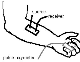
Fig. 3. Experimental arrangement in the forearm experiment. The sensor consisting of source and receiver fibers is placed along the radius. Pulsation is monitored by a pulse oxymeter probe placed at the ring finger tip.
