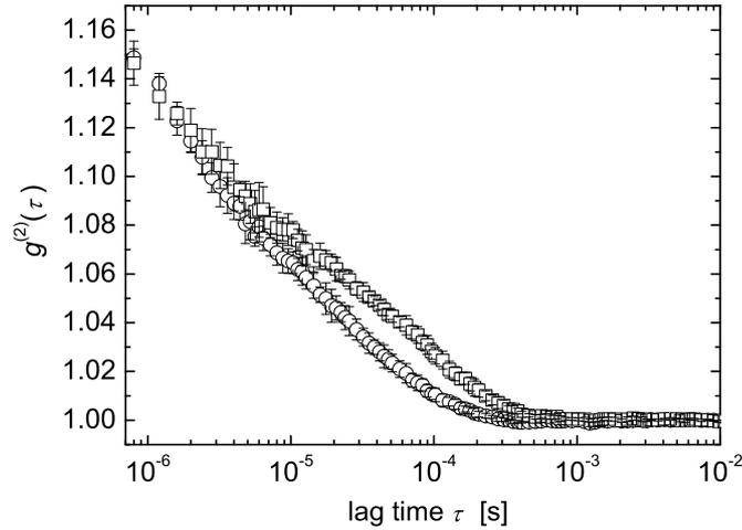
Fig. 6. Intensity autocorrelation functions  $g^{(2)}(\tau)$  recorded on the wrist for a systolic phase (time = [850, 1050] ms, circles) and a diastolic phase (time = [1250, 1450] ms, squares). The error bars represent the standard deviation over 5 repeated measurements. The source-receiver distance is 2.3 cm.
