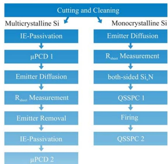
**Figure 1:** Processing sequence applied to mono- and multicrystalline samples for lifetime and emitter saturation current density measurements.
