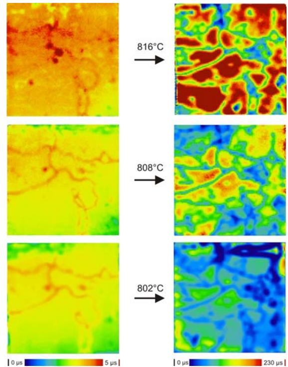
**Figure 4:** Minority charge carrier lifetime maps of neighbouring mc Si wafer before (left) and after (right) different  $\text{POCl}_3$  emitter diffusions at different temperatures. Surface passivation was enabled using an IE solution.
